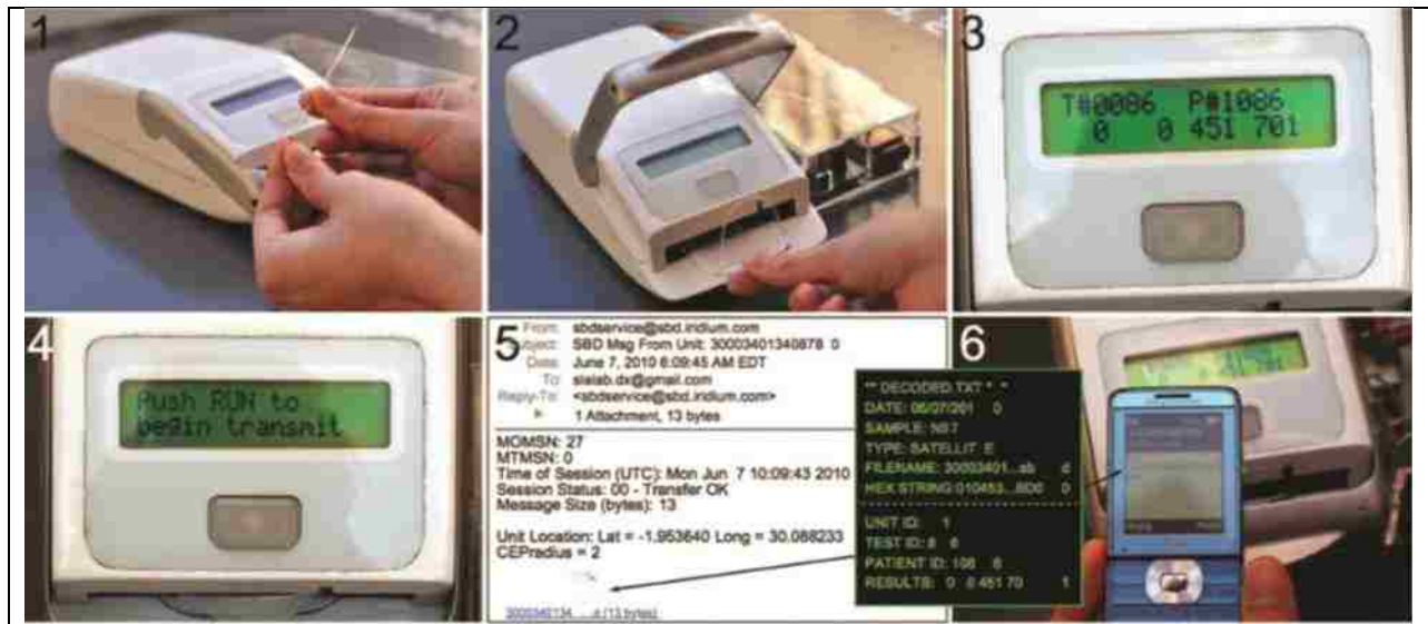
Figure 18: The fully integrated mChip system from the Sia group.[60]. This device plus- chip system performs ELISA-like diagnosis of HIV from 1 mL of whole blood and transmits the result to the patient's electronic health record stored on the cloud. Figure from Chin et al., Mobile Device for Disease Diagnosis and Data Tracking in Resource-Limited Settings, Clin. Chem., 2013, 59, 629–640. Figure reproduced from the American Association for Clinical Chemistry.
