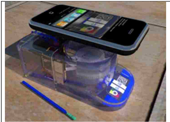
Figure 1: MAD NAAT device. Swab sample obtained from the patient is inserted in the device. The automated assay quantifies nucleic acid sequence of interest. After some time, the cell phone quantifies assay signal. Graphic by Paul Yager.
