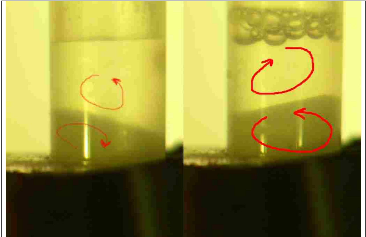
Figure 53: Comparing AudioLyse bead slurry movement with (right) and without (left) micro90 surfactant. The only superficial difference apparent in the videos was the presence of the bubbles at the top of the tube with the micro90, present due to vibration while the magnet, beads, micro90 and water were added.
